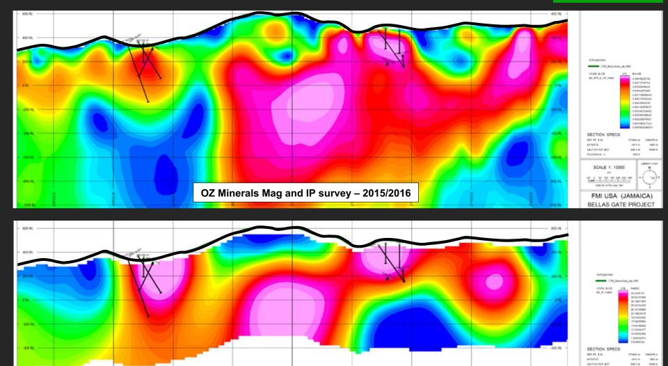
Mag and IP Converge with Depth, Interpreted Bornite-Core
