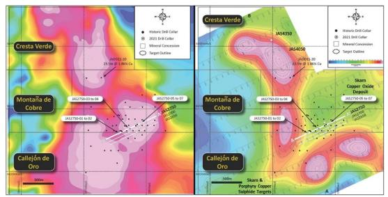
Figure 3 – Magnetics Analytical Signal Image (left); IP-Chargeability (right) over drill permit area.
