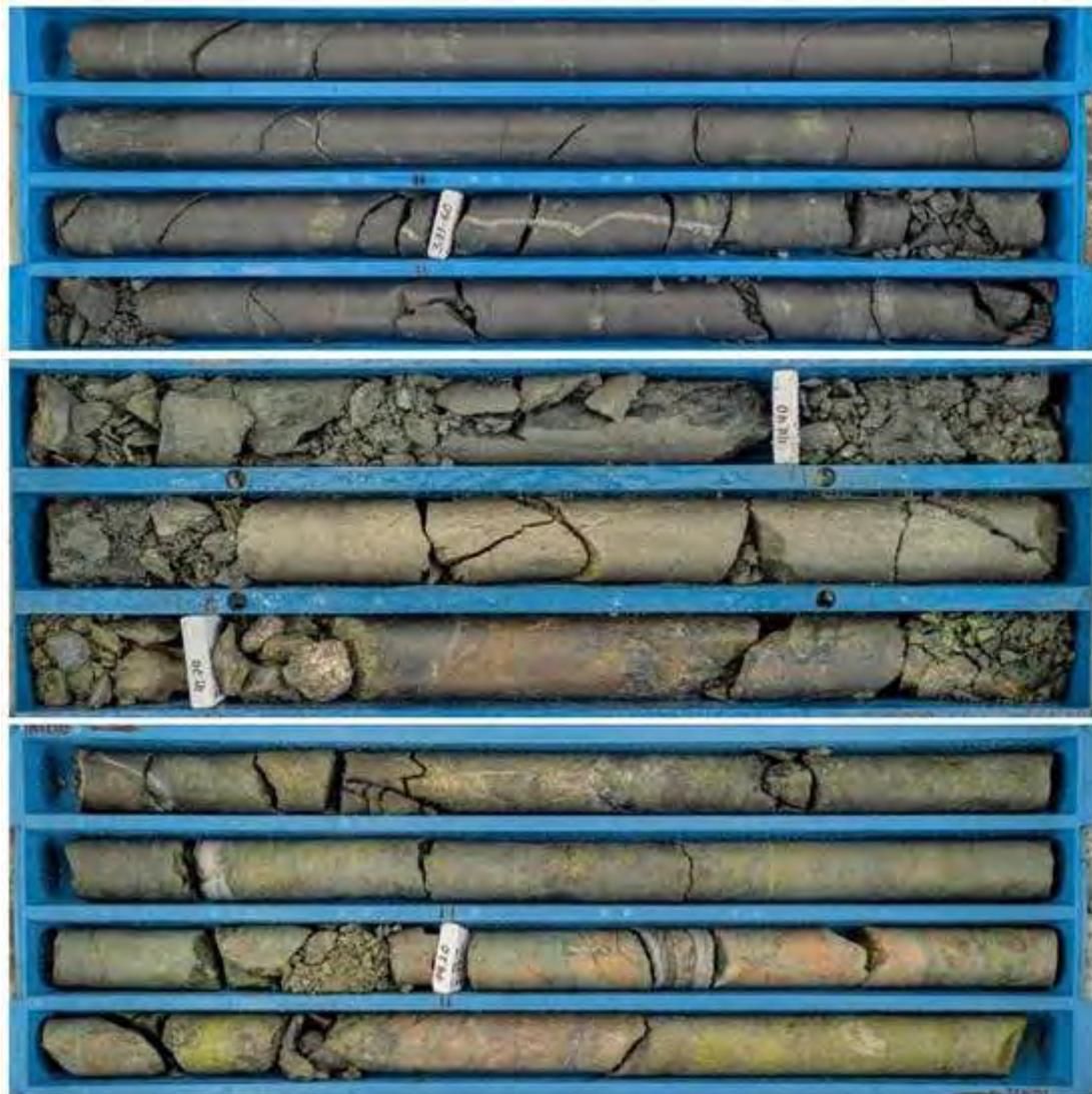
Figure 7 – (Top) KHZ5825-003 Massive magnetite skarn cut by quartz-chalcopyrite-bornite veinlets and with disseminated chalcopyrite. The 1.7m interval assayed 0.67% copper, 0.063 g/t gold, 1.82 g/t silver and 122 ppm molybdenum from 370.9m to 372.6m downhole depth. (Middle) KHZ5790-001 Garnet-diopside skarn cut by pyrite-chalcopyrite mineralization. The 1.9m interval assayed 1.38% copper, 0.27 g/t gold, 7.14 g/t silver and 5 ppm molybdenum from 43.9m to 45.8m downhole depth. (Bottom) KHZ5790-001 garnet-diopside skarn with strong chalcopyrite mineralization, and cross-cutting quartz sulfides veinlets. The 1.4m interval assayed 4.91% copper, 0.42 g/t gold, 17.35 g/t silver and 164 ppm molybdenum from 77.1m to 73.5m downhole depth.
