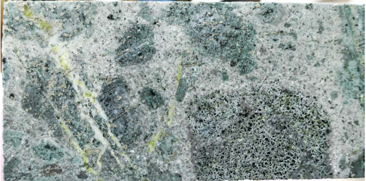
Figure 4: (TOP) CMH8350-001 at 175.9m, core interval 175 – 177m assayed 0.56% copper and 0.19g/t gold (0.69% CuEq 1 ). (BOTTOM) Vuggy residual quartz fragment in CMH8350-001 at 657.9m.
