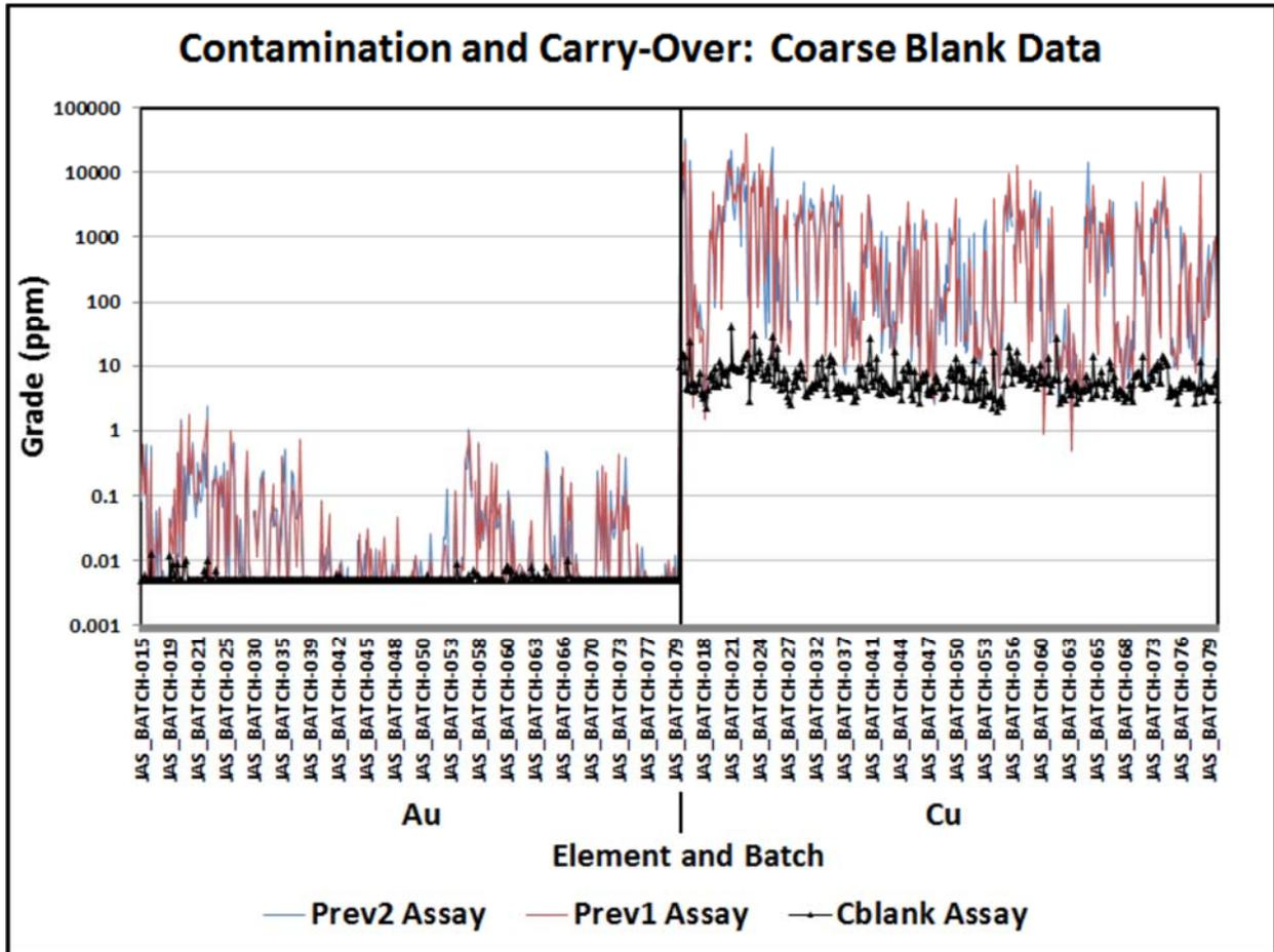
Figure 11-14. Coarse Blank QC Analysis – Phase 2 Drilling (Hackman, 2022)
