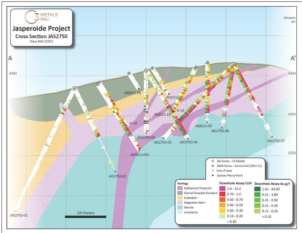
**Figure 10-9. Cross Section JAS2750 from Phase 1 Drilling with Generalized Geology and Historical Drill Holes with a ±50 m Window (C3 Metals, Inc.)**
