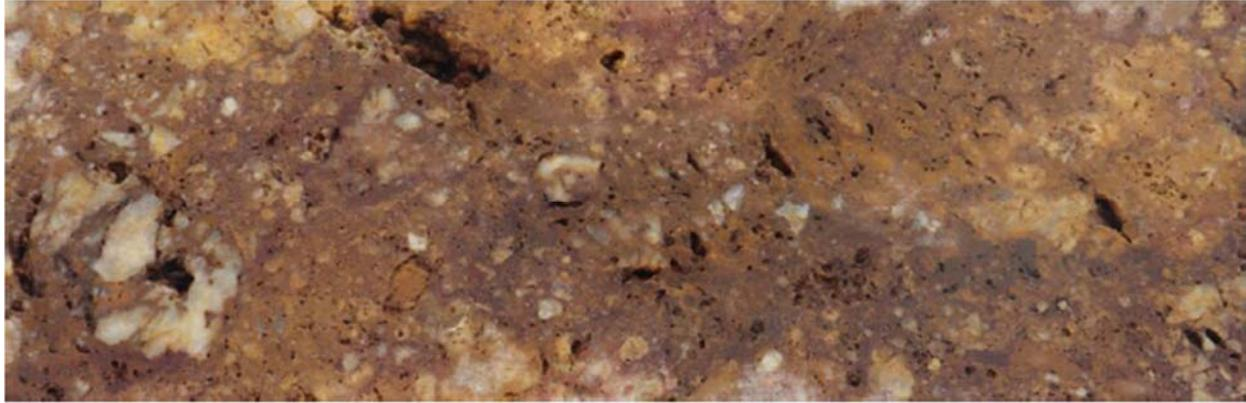
**Figure 10-8. Core from Drill Hole JAS2700-04 (~84.2 m) Showing a Vuggy and Intensely Silicified Polymictic Breccia which is Part of an Intercept that Assayed 0.13% Cu, 0.17 g/t Au and 2.44 g/t Ag over 29.7 m (from 70.3 to 100.0 m) (C3 Metals, 2021)**
