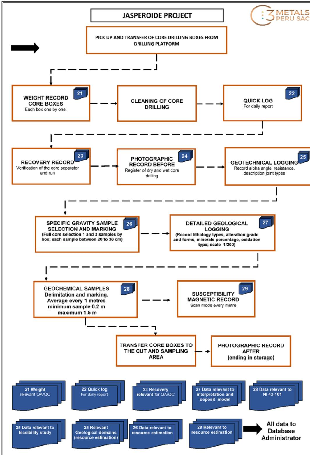
Figure 10-11. Flowsheet for Core Handling from Pick Up at the Drilling Platform to Final Sampling and Database Capture (C3 Metals, 2021)
