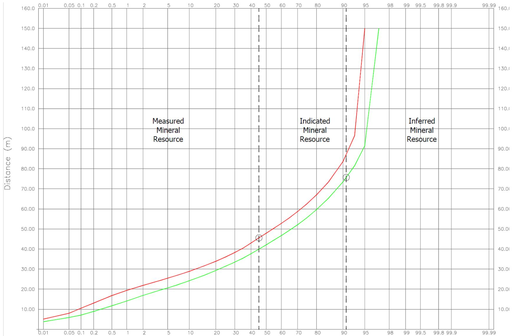
Figure 14-14. Probability Plot of Distance to Nearest 3 and 4 Holes for Altered Limestone (IMC, 2023)
