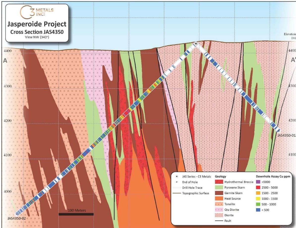
**Figure 10-10. Cross Section JAS4350 from Phase 1 Drilling (Cresta Verde Zone) with Generalized Geology and Historical Drill Holes with a  $\pm 50$  m Window (C3 Metals, 2021)**
