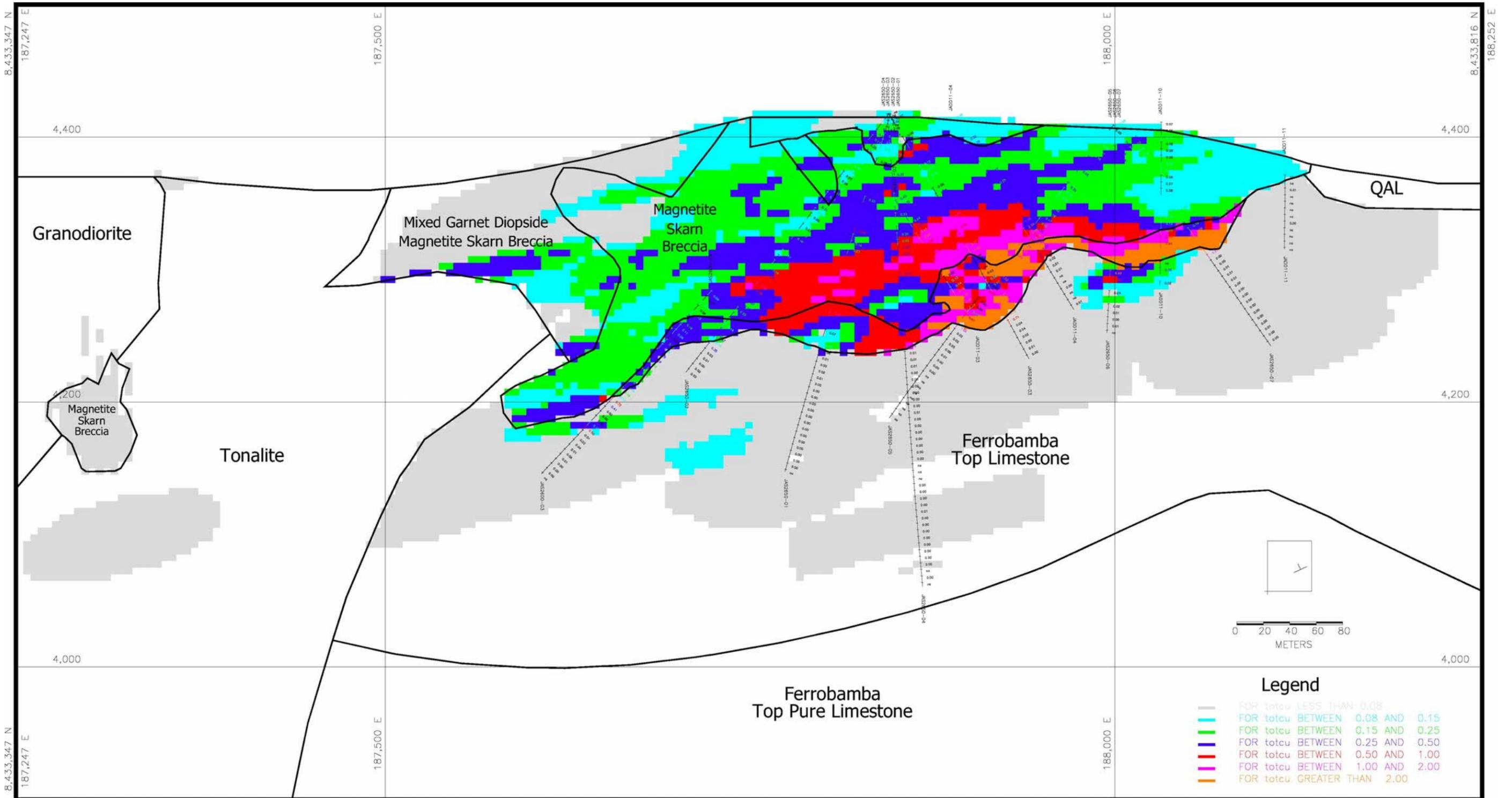
Figure 14-10. Copper Grades on Cross Section 2650 (IMC, 2023)
