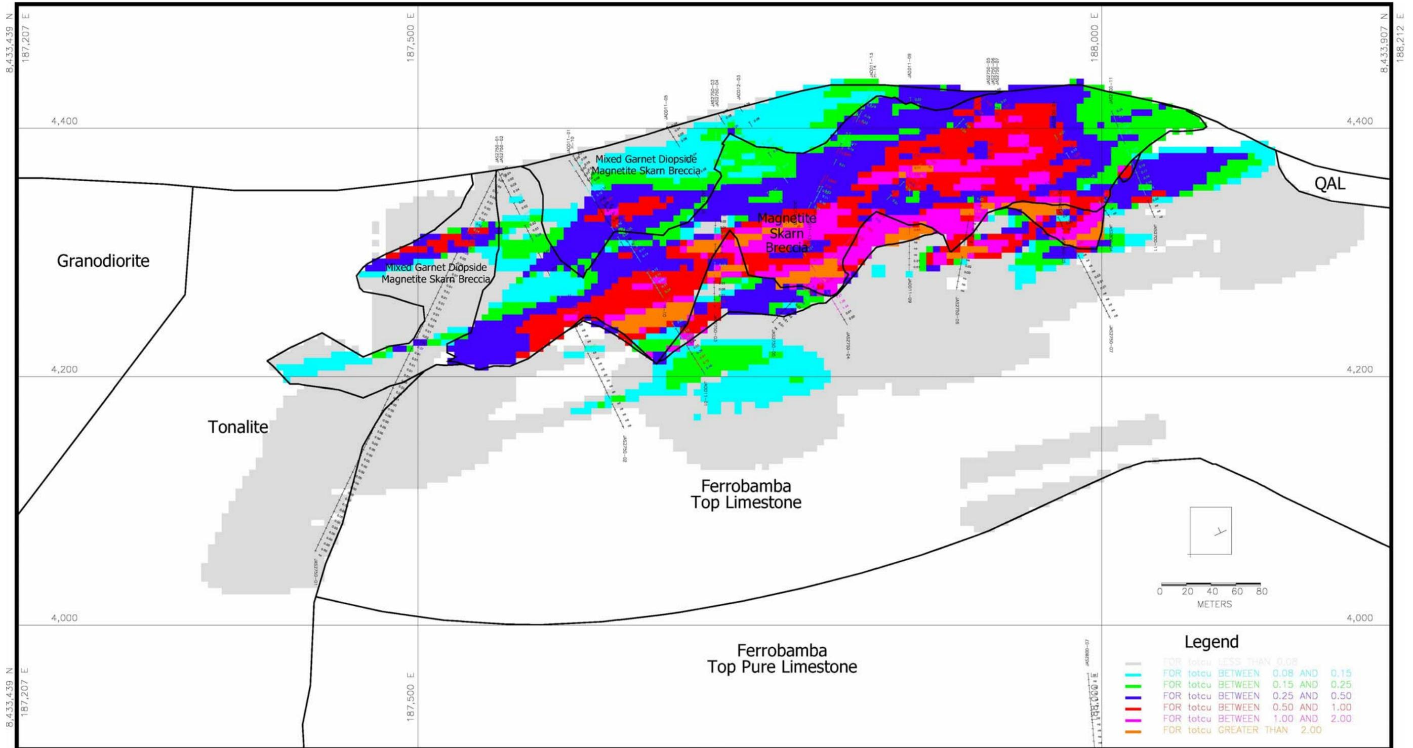
Figure 14-11. Copper Grades on Cross Section 2750 (IMC, 2023)
