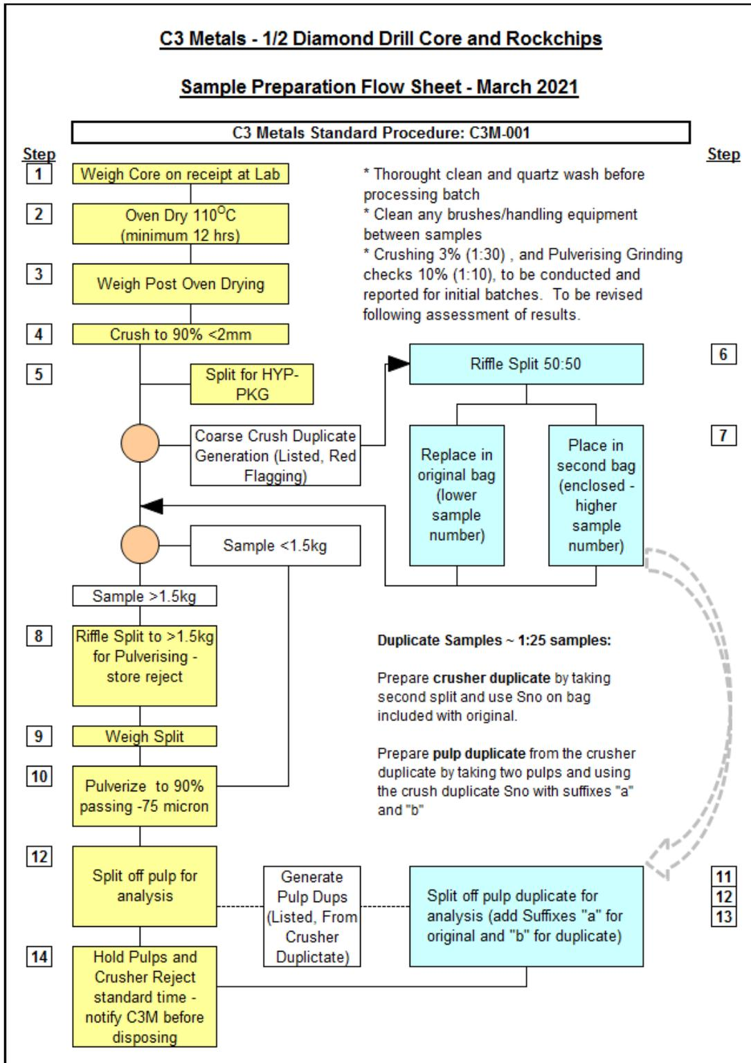
Figure 11-1. Sample Preparation Flow Sheet (C3 Metals, 2021)
