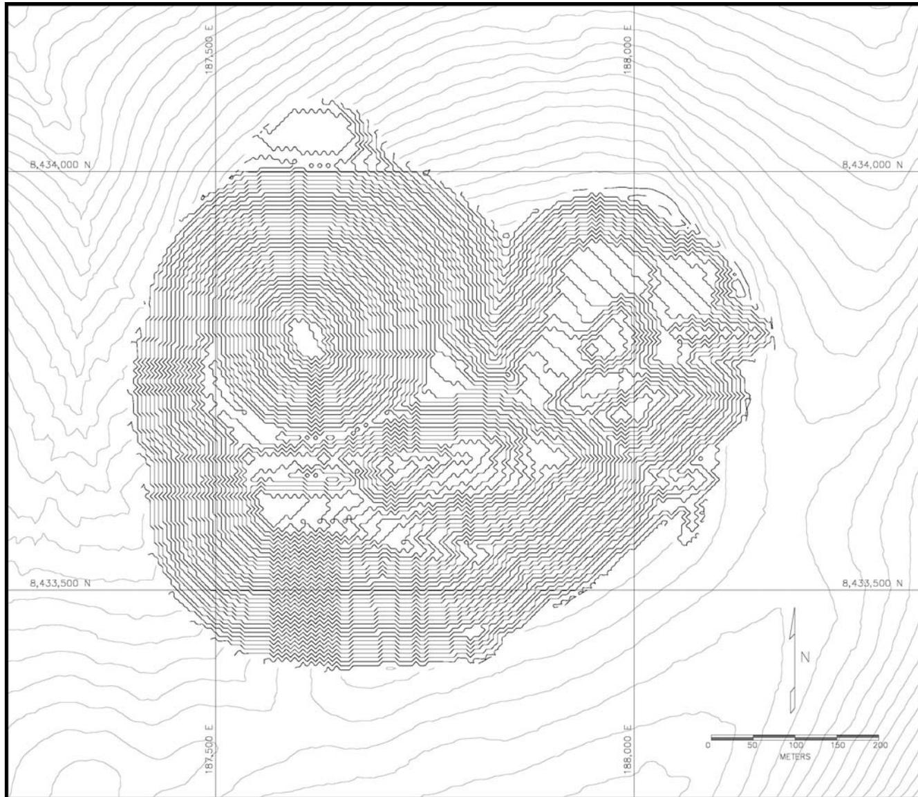
**Figure 14-1. Constraining Pit Shell for Mineral Resource Estimate (IMC, 2023)**
