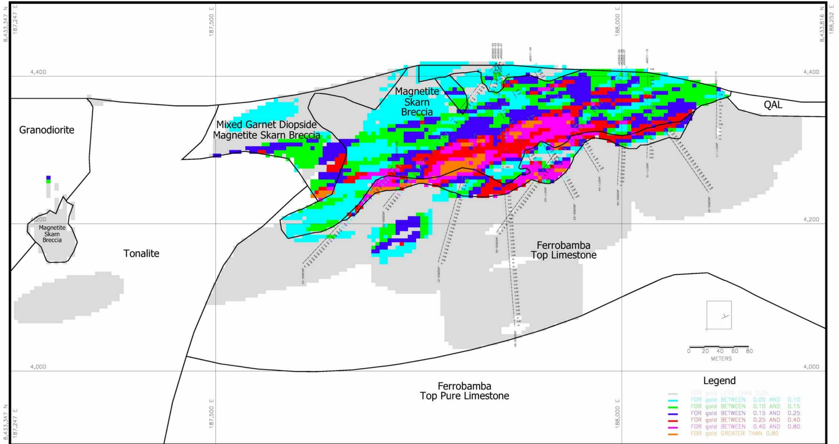
Figure 14-12. Gold Grades on Cross Section 2650 (IMC, 2023)
