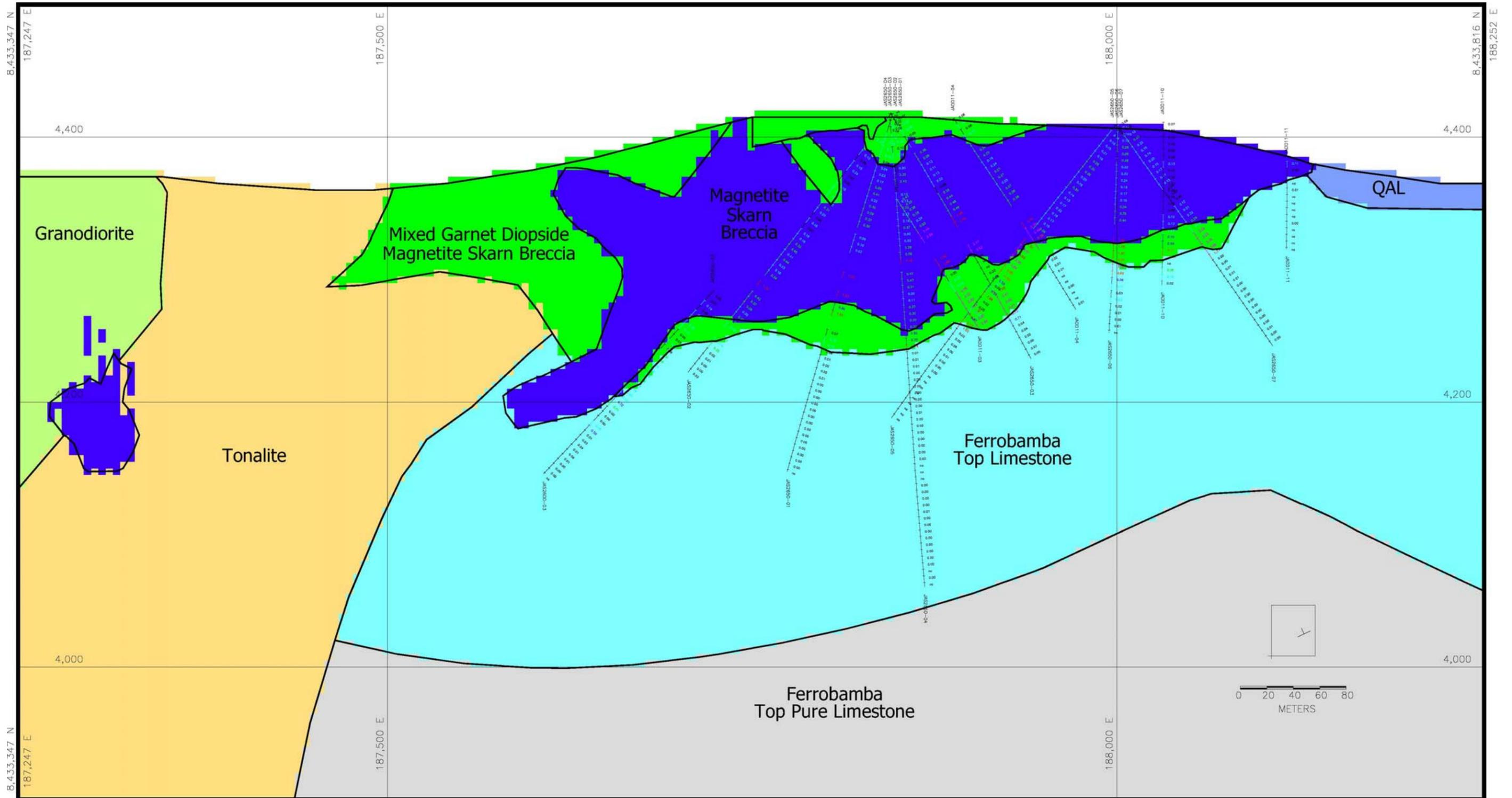
Figure 14-3. Rock Types and Alteration Types on Section 2650 (IMC, 2023)
