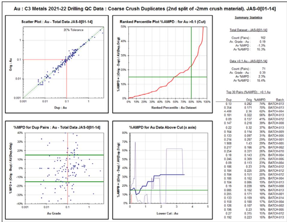
Figure 11-11. Au in Coarse Crush Duplicates (Hackman, 2021)
