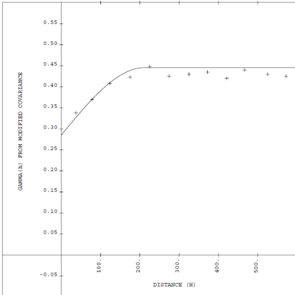
Figure 14-9. Copper Variogram Along Minor Axis (IMC, 2023)
