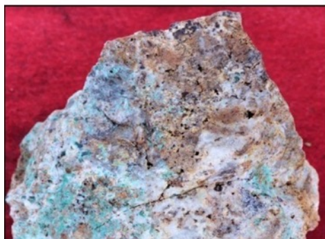
Epithermal quartz breccia assayed 2.60% Cu, 6.0g/t Au
