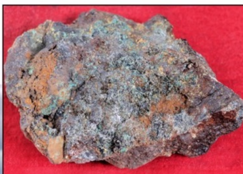
Skarn with bornite assayed 2.61% Cu, 0.11g/t Au
